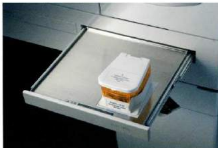
The cassette is recognized with RFID. (PAT. P)
